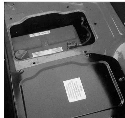
Rubber bumper cars have a single 12 volt battery as shown here. This battery has a red protective cover over the 12 volt i.e. positive terminal and connector of the battery.
