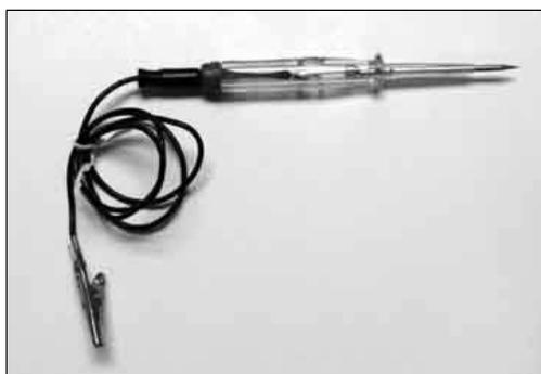
One of the first difficulties is that different faults require different types of measuring kit. Sometimes there is an overlap and in most cases a test-light will work as well as a meter. This is a small 12 volt bulb or LED, inside a probe similar to a screwdriver, with a point at one end and a wire with a crocodile clip at the other. Or it could simply be a spare
