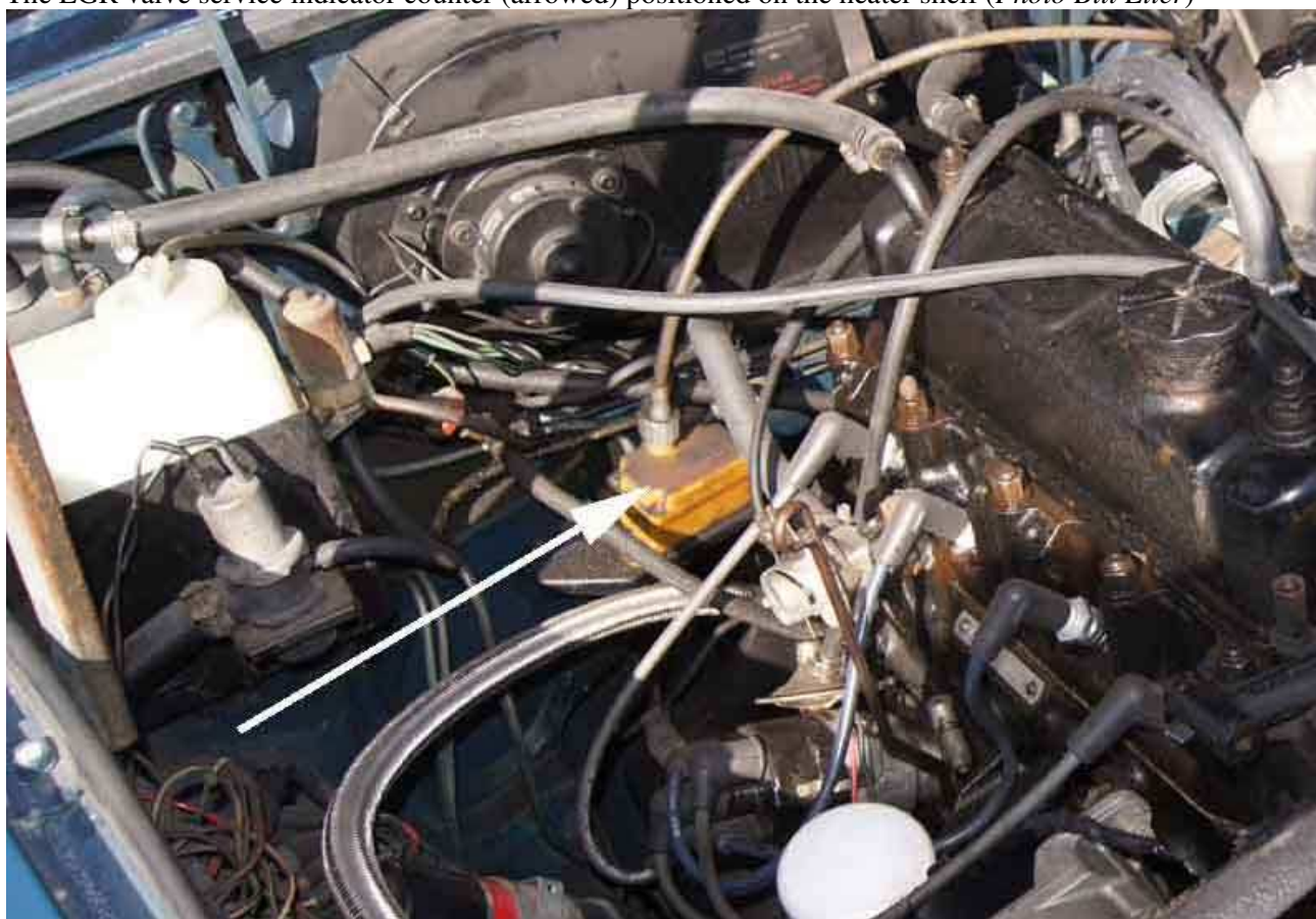
The EGR valve service indicator counter (arrowed) positioned on the heater shelf ( Photo Bill Etter )
