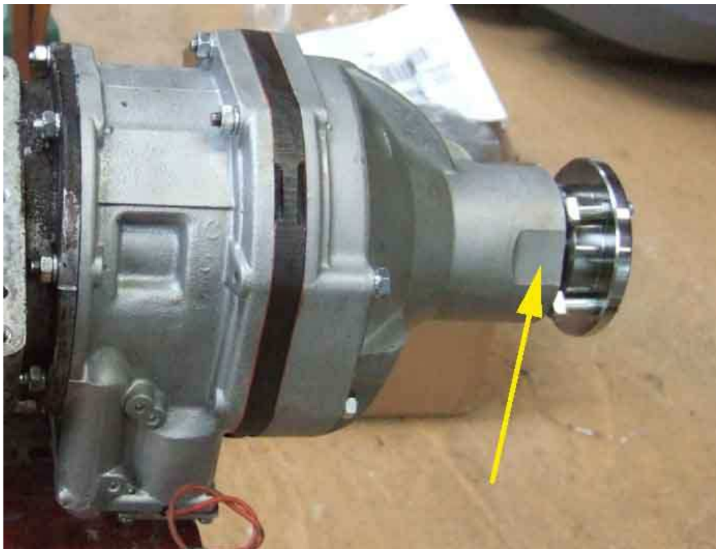
The 4-cylinder has a smaller flange and as shown by the arrow the flat on the bolt doesn't even clear the oil seal
