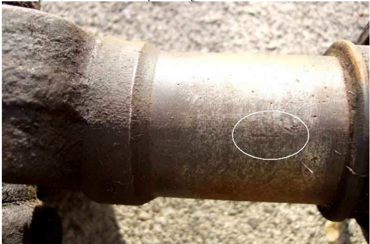
My old V8 shaft, two lines on the yoke, which could be the shaft and half of a detached head, but nothing on the tube. These are also sort of but not exactly in-line with one of the arms of the yoke, and not between them as on Fletcher's so could be nothing at all, but are close to the example bottom right above.
