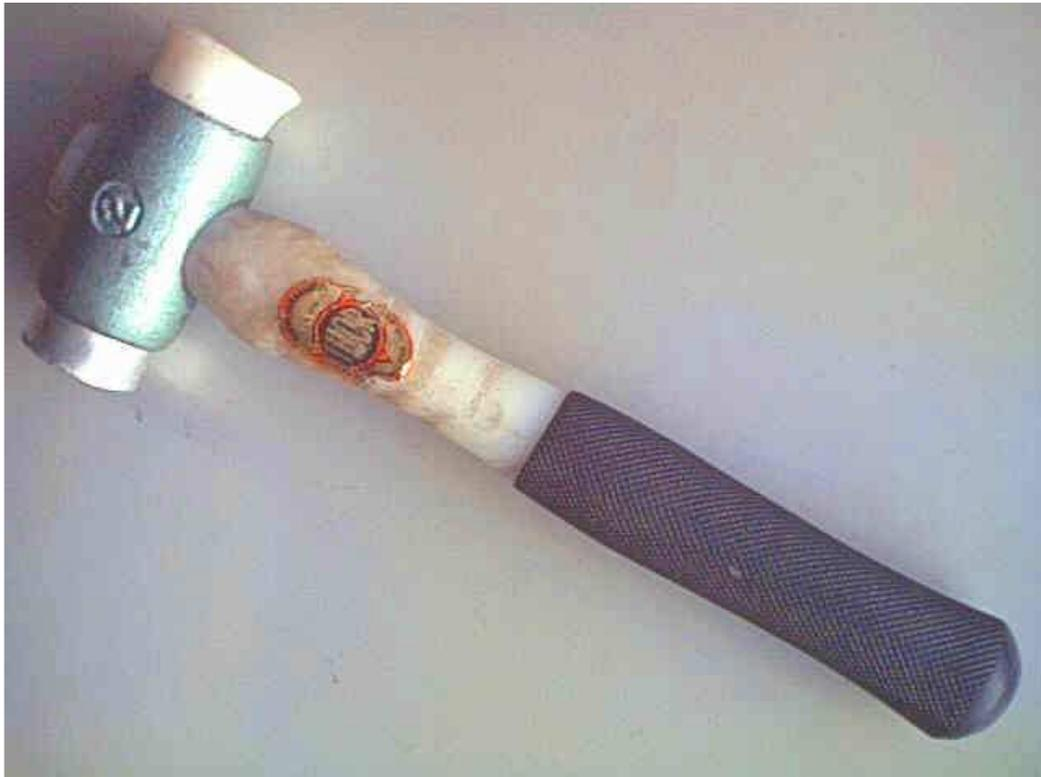
My preferred Thor hammer with a nylon insert one end. This has deformed slightly over the years but hasn't marked the spinners at all.
