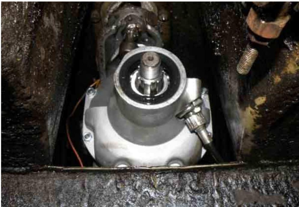
The 'ice pick', and the large socket that was used to drift the new seal into position
