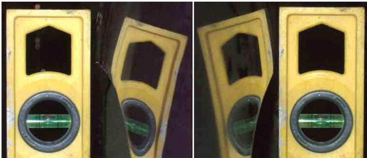
The shape of the reflection also shows how there is more of a curve below the trim strip on the left compared to the right. This puts the trim strip on the left another 6mm further away from the spinner compared to the right, making a 12mm or nearly half an inch difference between sides, if both wings had the same profile.
