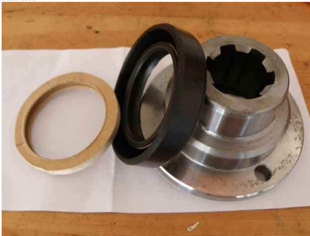
The seal fitted over the flange
